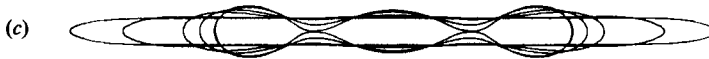
FIGURE 9. Relaxation and breakup of low-viscosity-ratio droplets in an otherwise quiescent fluid; \lambda = 0.01 . The initial shape is taken from an experiment for \lambda = 0.011 . Low-viscosity-ratio droplets have long, slender shapes with nearly pointed ends. (a) L/a = 5.3 ; (b) 6.4; (c) 7.5. Successive times t are shown on the figure.
