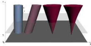
Fig. 2: Models of the future (from left to right): fixed object (1); moving object with constant velocity (known future motion) (2); conservative models for a moving point with unknown future motion and upper-bounded velocity (3), and upper-bounded acceleration (4).
