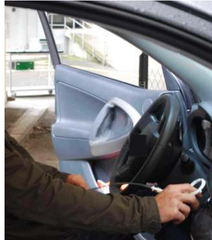
(b) Starting the engine using the relay.
