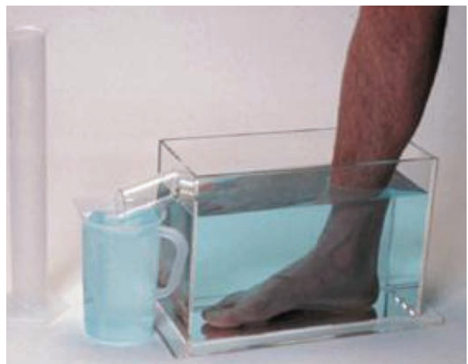
Figure 3. Baseline volumeter measuring device, foot set, 5x13x6 inches (reproduced with permission from WisdomKing.com).
