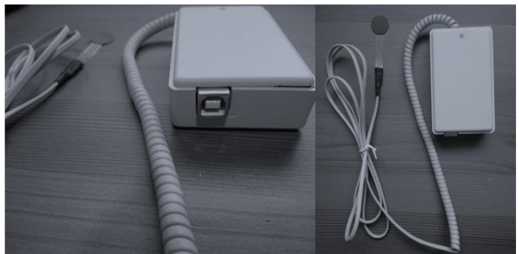
Figure 1. Prototype tongue force device (inferior and upper views). Small casing protecting the backplane, extralong cable, and piezoelectric sensor.
