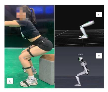
**Figure 1.** (**A**) Photograph of a participant wearing reflective markers and the Perception Neuron<sup>®</sup> device during a squat trial. (**B**) A screenshot of the software program that was used to obtain motion data information from the OptiTrack device. (**C**) A screenshot of the software program that was used to obtain motion data information from the Perception Neuron<sup>®</sup> device.
