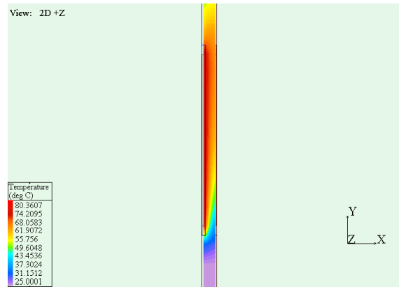
Fig. 5 Temperature distribution in channel between fins
