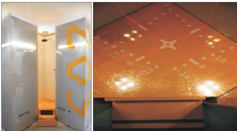
Fig. 2. EOS system cabin to scan the patient in a standing position in two orthogonal planes.
