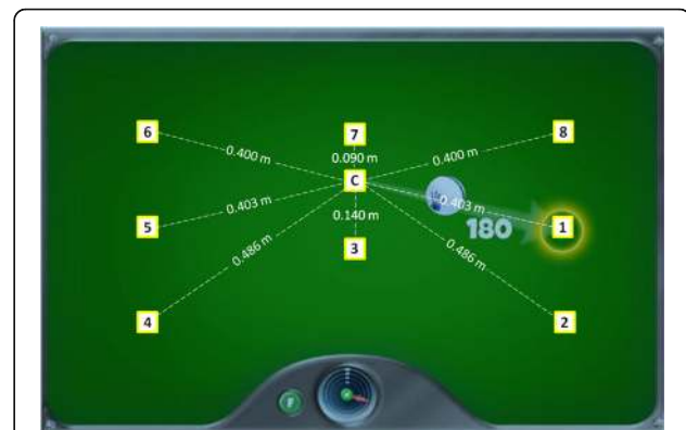
Fig. 2 The evaluation task of MOTORE. In figure is showed the visual feedback showed to the patients on the screen, together with the position of each target. The white ball indicates the position of the end-effector; the yellow circle indicates the target to be reached. The yellow squares, not showed to the patient during the task, indicate the position of the targets: C is the central target, while the numbers from 1 to 8 indicate the external targets with the sequence of the center-out movements. In addition, the distance of each target from the center is reported
