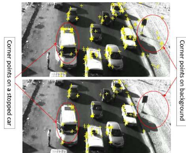
FIGURE 5. Example of excluding the corner points in the background while retaining the corner points of stopped vehicles. The top frame presents all corner points, and the bottom frame presents the corner points after excluding the points in the background.
