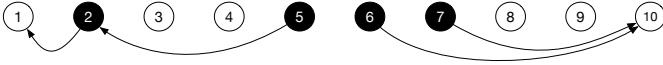
Figure 7. Example with a policy X over n = 10 destinations, with K = 4 destinations (2, 5, 6 and 7) having lost a packet. Arrows indicate recovery requests (SR-NACKs): destination 2 requests recovery from peer 1; destination 5 from peer 2; and destinations 6 and 7 from peer 10; S_X = 3 recovery requests are successful ( i.e. , those from 2, 6 and 7), as peers 1 and 10 have correctly received the original packet; T_X = 2 retransmissions are performed (from 1 and 10).
