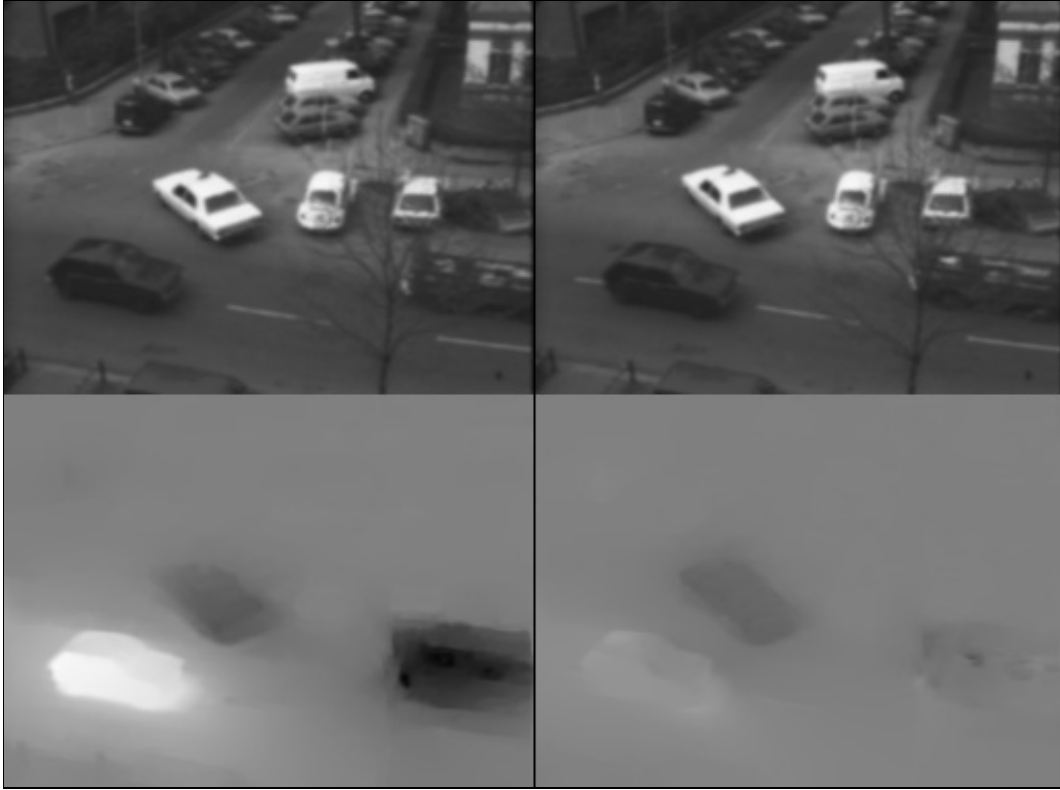
Figure 4: Computation of the optical flow for the taxi sequence (frames 15 and 19) with \alpha = 0.6 , s = 0.1 , \sigma_0 = 10 , \sigma_n = 0.8 , and \eta = 0.95 .
