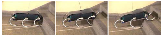
Figure 12 – ‘First step’ algorithm. Left: robot stands before flight. Center: front left leg recirculates and pulls RHex onto first stair. Right: Front right leg recirculates so that RHex is posed to enter the stair climbing algorithm.
