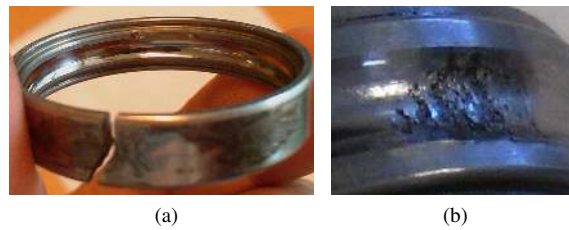
Fig. 8: Failure of the bearings of Pronostia: (a) extern ring failure, and (b) inner ring failure.
