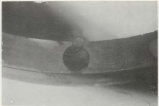
Fig. 5(a) Crack in compressor spacer
