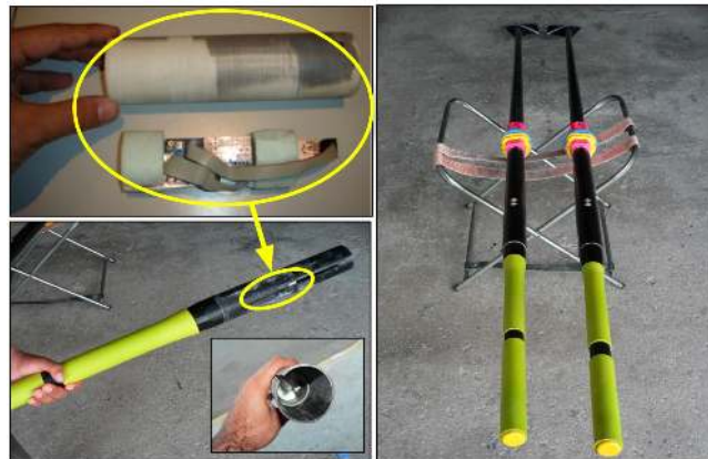
Figure 4. Mounting the mote inside the oar.
