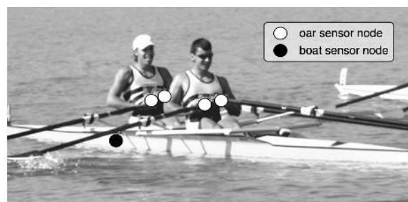
Figure 1. Position of the sensor nodes on the boat.
