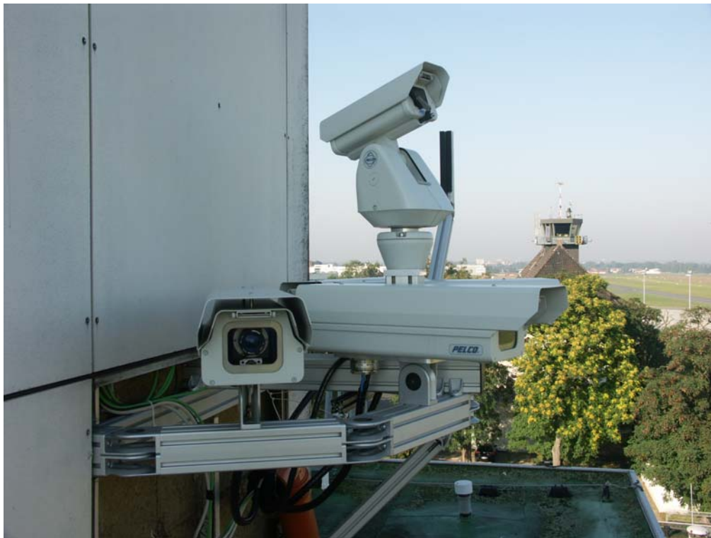
Fig. 5: High resolution panorama camera setup and pan-tilt zoom camera of the video panorama system. Braunschweig tower in the background (Photo DLR).
