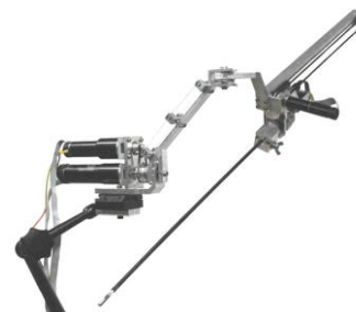
Fig. 5 Overall figure of the 5-DOF spherical mechanism surgical robot, CURES
