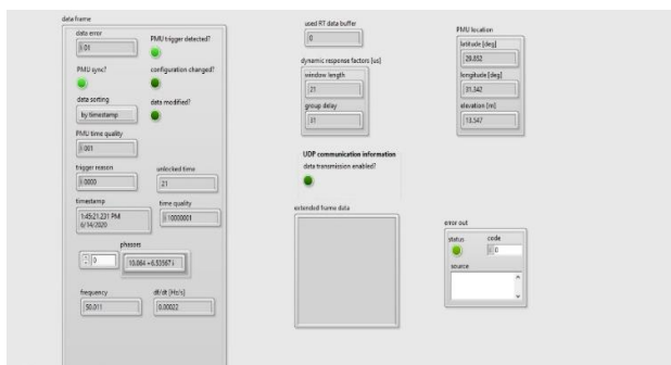
Fig. 9 Phasor Measurement Unit Output Data
