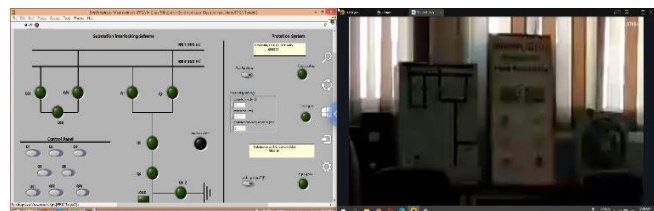
Fig.7 Interlocking Schemes Using LabVIEW for Double Bus Bar Single Breaker Substation Scheme and View from the Lab.
