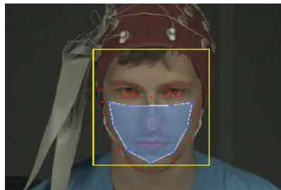
Figure 2. ROI detection and tracking. The yellow line shows the face rectangle, inside which feature points are detected and tracked. The red points indicate 66 landmarks and the light-blue region is the defined ROI.
