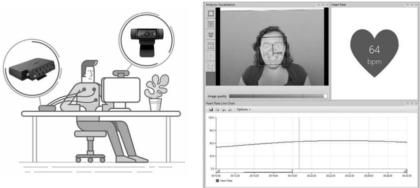
Fig 1. Experimental setup and software. On the left, a schematic representation of the experimental setup and the devices: ProComp Infronti T7500M (ECG recording) and Logitech HD Pro Webcam (video acquisition). On the right, a screenshot of the Facereader rPPG software by Noldus.
