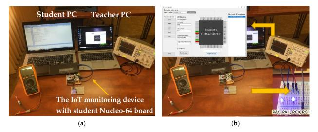
**Figure 10.** (a) Workplace of a remote laboratory with a teacher PC, a student computer, and the IoT monitoring device with measuring devices (multimeter and oscilloscope). (b) GPIO pins monitoring where PA0, PA1, PC0, and PC1 pin was tested.
