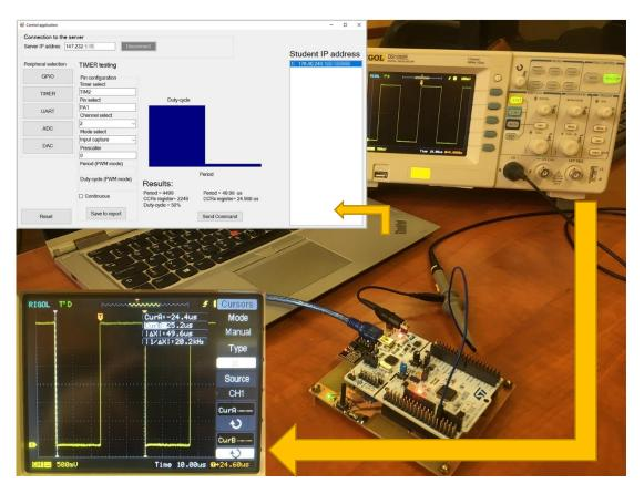
**Figure 11.** PWM monitoring provided by timer TIM2. The oscilloscope captures the signal showing 50  $\mu$ s periods with 50% duty-cycle. The results are shown in the upper left corner of the control application.
