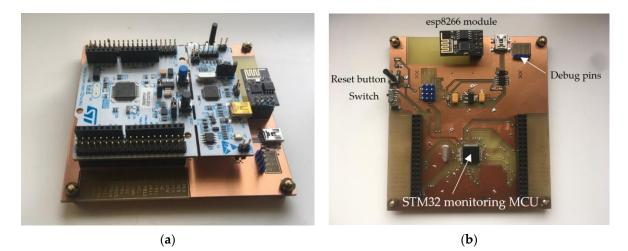
**Figure 3.** A hardware part of the IoT remote laboratory: Student Nucleo-64 board connected to the IoT monitoring device (**a**) and created PCB (**b**) with equipped monitoring microcontroller STM32F446RE, IoT module esp8266, and the other required components.
