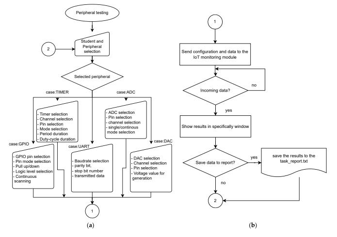
**Figure 6.** The shown flowcharts mainly create control application functions. The first part marked as (a) describes the selection of the tested peripherals and the manual input of peripheral configurations, or the selection of data sent to the server and subsequently to the IoT monitoring device. The (b) is a continuation of the first part of the algorithm, which describes the method of receiving the response from the IoT monitoring device, its display and storage in the report.
