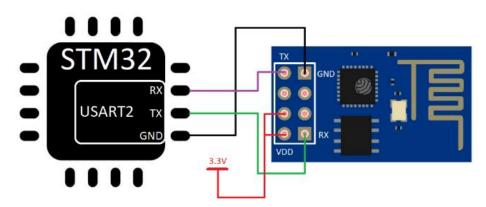
Figure 8. Monitoring STM32 microcontroller and esp8266 module connection via USART2.
