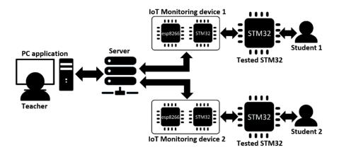
Figure 2. The IoT remote laboratory design in blocks.
