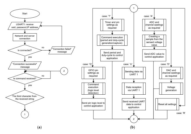
**Figure 7.** The last flowchart shows how the IoT monitoring device works. The flowchart consists of two parts, where (**a**) is the first part and (**b**) is the continuation or the second part.
