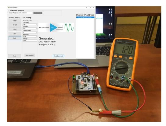
Figure 14. DAC testing with 12-bit DAC1, channel 1 generated through PA4 pin.
