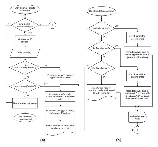
**Figure 4.** The shown flowchart describes the server program operations from the start of the server up to received data processing. The first flowchart (**a**) describes how clients connect to the server and save the data to a text file. The second flowchart marked as (**b**) is part of the first flowchart where the block "The other data processing" is extended and described.
