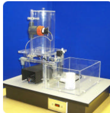
Figure 2. Variable speed pump-flow-level station
