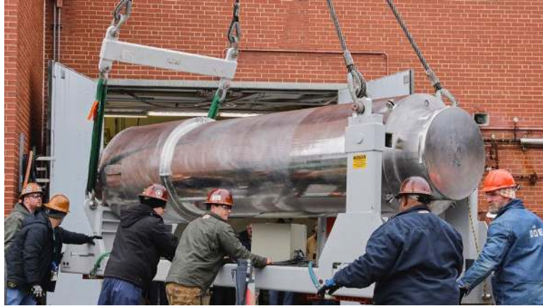
Figure 10. Used nuclear fuel cask at ORNL (ORNL photo 2016-P00292).
