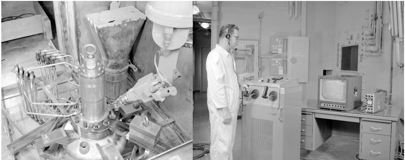
Figure 1. Manipulator arm and pump in hot cell (right) and controlling manipulator via camera and monitor (left) (ORNL photos 42878 and 43068 both from ORNL-CF-58-4-93).
