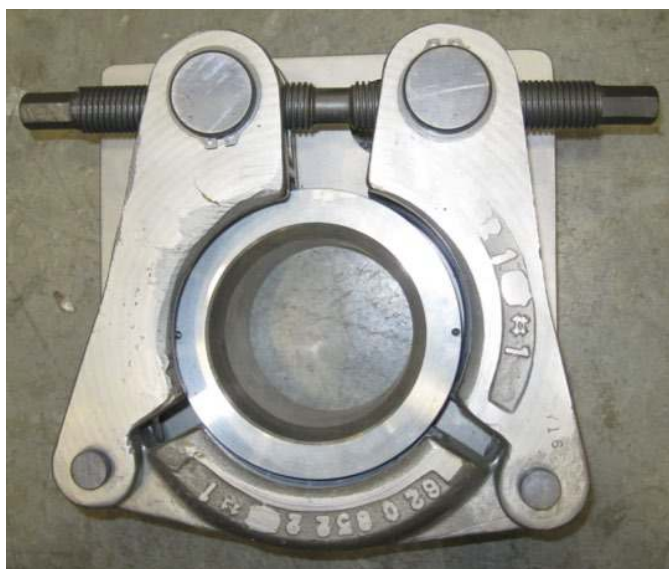
Figure 11. Graylock flange for remote operation (photograph taken by author).
