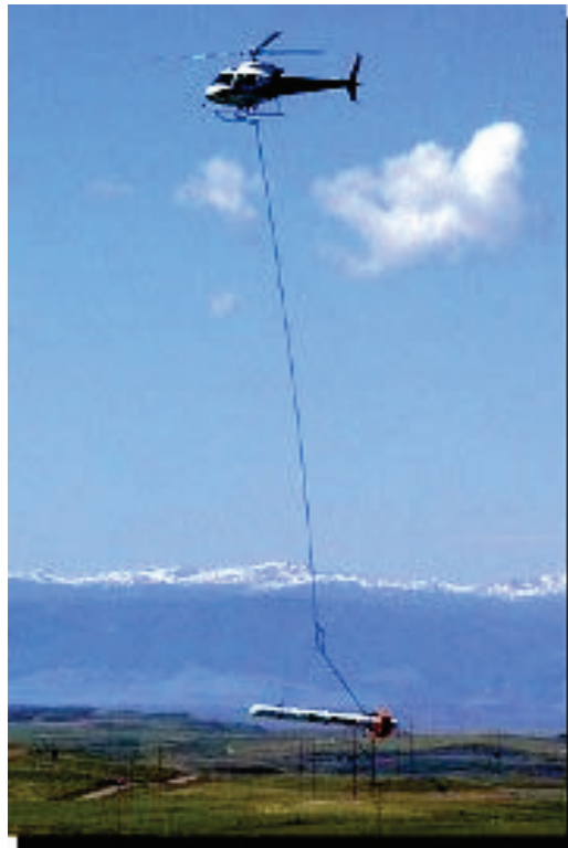
Figure 6-2. An airborne EM survey being conducted showing the towed EM “bird.”
