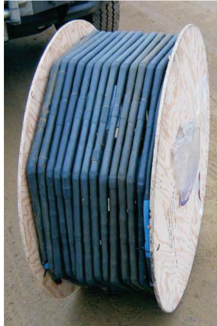
Figure 5-14. SAA on shipping reel (32 mm) (Abdoun and Bennett 2008).
