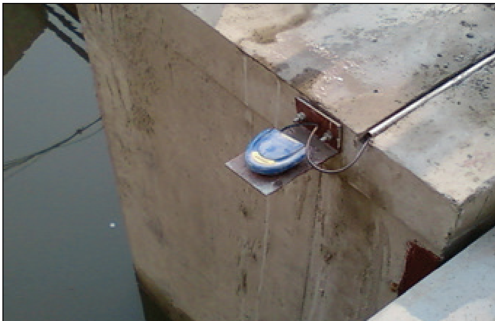
Figure 5-50. Ultrasonic level sensor: EchoSonic II (Flowline 2011).
