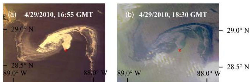
Fig. 2 MODIS RGB images (R: 645 nm; G: 555 nm; B: 469 nm) showing oil slicks with different optical contrast (spectral reflectance) only 1.5 h apart, due to different solar/viewing geometry and wind. (a) April 29, 2010, 16:55 GMT and (b) April 29, 2010, 18:30 GMT. The image width is about 120 km. The red X shows the DWH spill location. Figure adapted from Hu et al. 27
