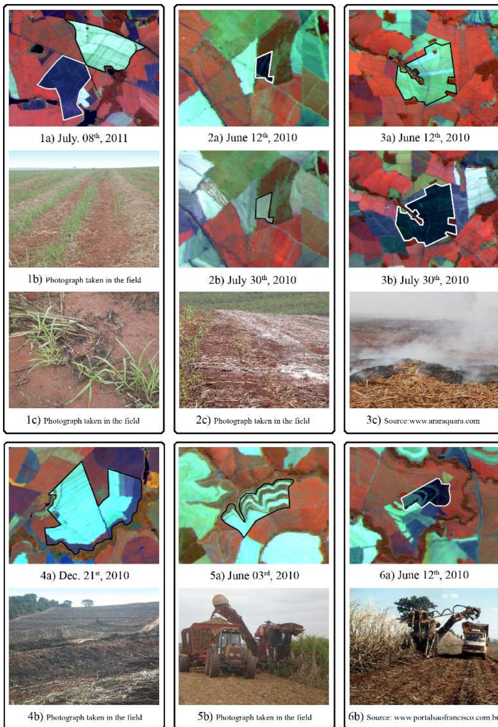
Figure 2. Multispectral [4(R)5(G)3(B)] and multi-temporal Landsat-5 images illustrating some instances in which post-harvest management influences the correct identification of sugarcane as either green harvest (GH) or pre-harvest burning (BH). GH and BH (1a); BH (2a) with later application of lime on top of the soil (2b and 2c); GH (3a) with the later burning of cane litter (3b); harvest in fields with slope \leq 12\% and with slope > 12\% (4a); GH with combiner (5a); BH with combiner (6a and 6b). Photos taken in the field (1c, 2c, 4b and 5b) and acquired on the Web for illustration purposes (3c and 6b).
