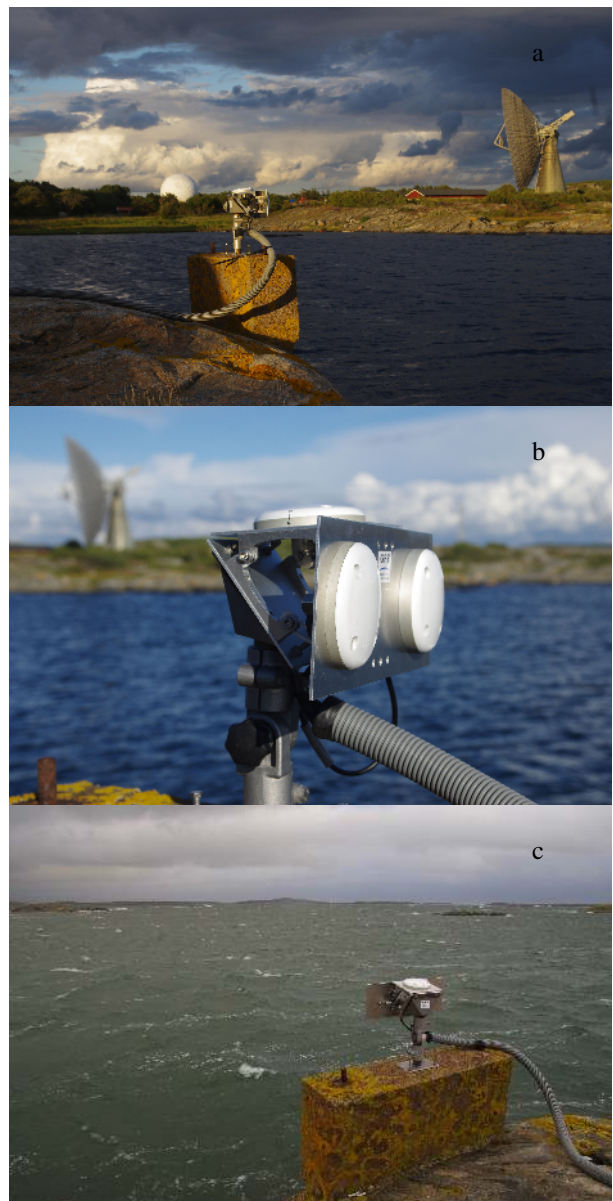
Fig. 5: An eastward view of the GFZ GNSS-R station at Onsala Space Observatory (a), the zenith looking, RHCP, and side looking, RHCP and LHCP, antennas (b), and the sea targeted at the antenna boresight (c).
