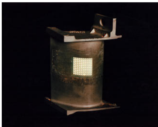
FIG. 26. Photograph of the heat-flux range gauge attached to a turbine blade.
