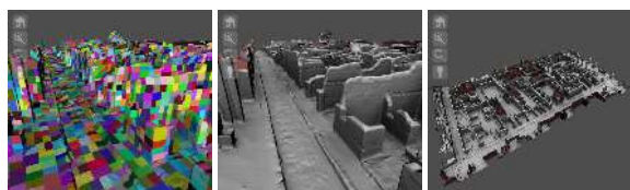
Figure 1: The multiresolution Engine. On left: the patches used, smaller and more detailed near the camera, larger and at a lower-resolution farther away. Middle: when rendering, the geometry appear as a continuous surface. On right: the multiresolution easily manage the whole 27 million triangles model of the Pompeii Insula.
