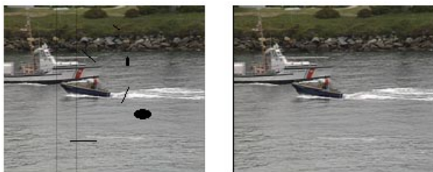
Figure 6. Performance of the complete restoration chain: Left: Blotch and line scratch degraded frame; Right: Restored image
