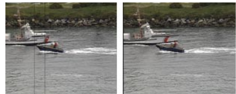
Figure 5. Performance of the LSSI interpolator: Left- Line Scratch degraded image; Right- Restored image
