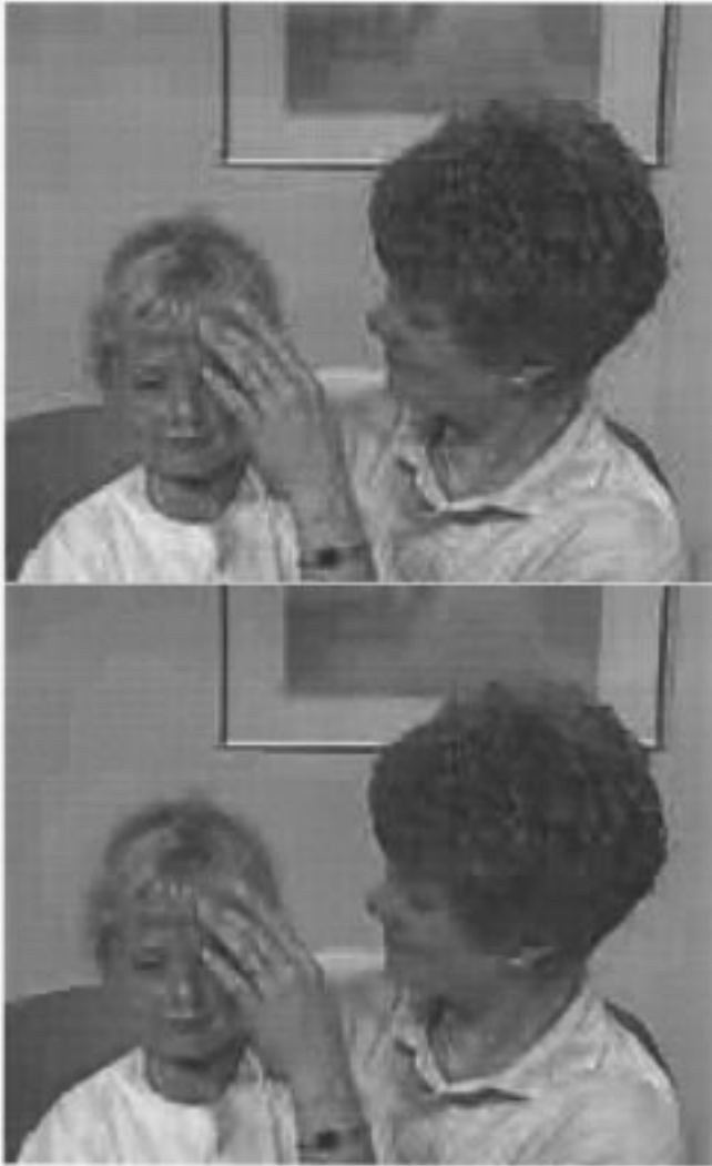
Fig. 3. “Mother and daughter” frame 21: MPEG compressed image (top); POCS reconstructed image (bottom).
