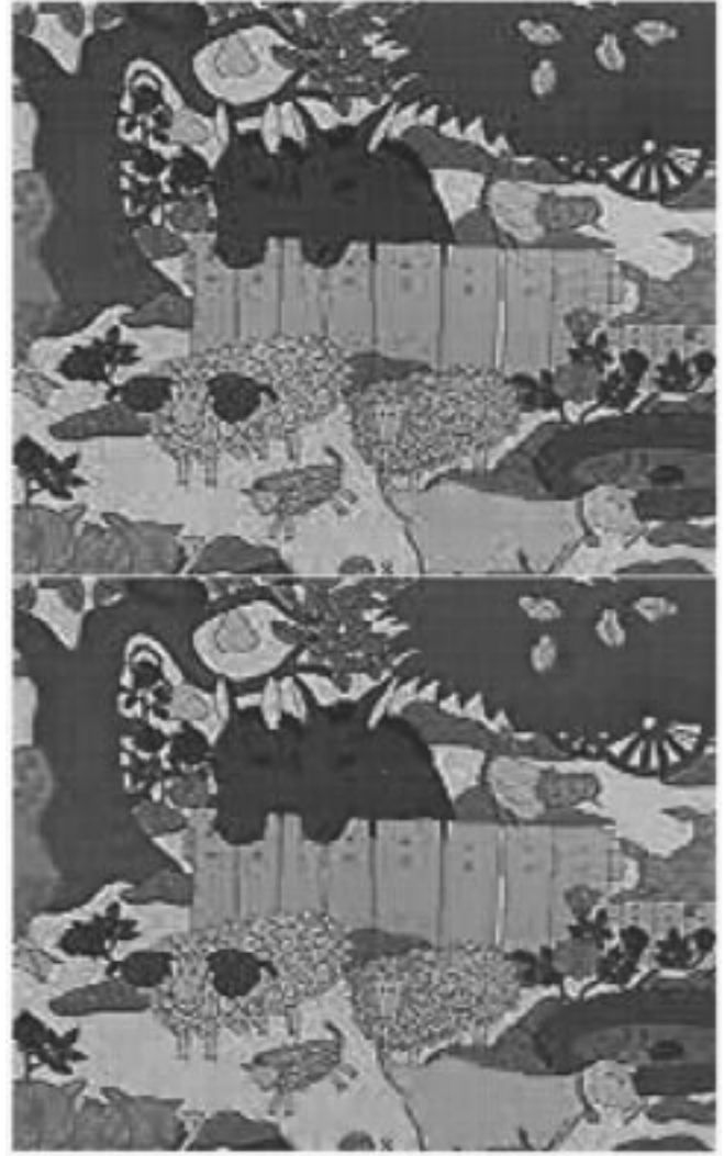
Fig. 6. "Mobile" frame 31: MPEG compressed image (top); POCS reconstructed image (bottom). Note that only a 176 \times 144 segment of the whole image is shown here.
