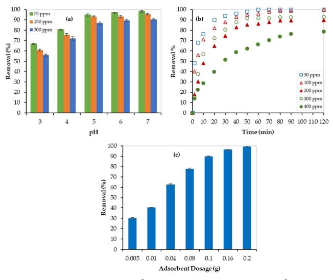
**Figure 7.** Removal of Pb<sup>2+</sup> by PEI/GO at 23 °C: (a) effect of pH, (b) effect of Pb<sup>2+</sup> initial concentration and contact time, and (c) effect of adsorbent dosage.
