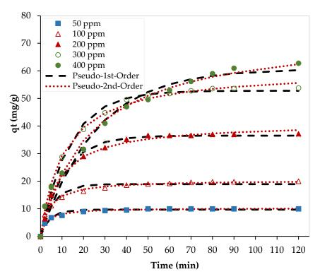
**Figure 8.** Nonlinear kinetic models. (pH = 6, PEI/GO dosage = 0.1 g, and 23 °C).
