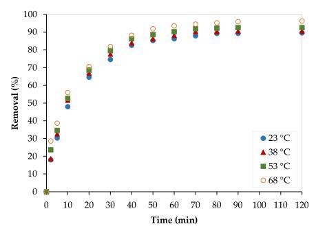
**Figure 13.** Temperature effect on the  $Pb^{2+}$  removal by PEI/GO. (pH = 6, PEI/GO dosage = 0.1 g, and  $Pb^{2+}$  initial concentration = 300 ppm).
