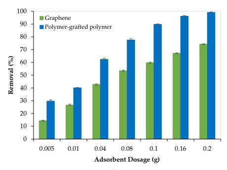
**Figure 6.** The removal performance of  $Pb^{2+}$  from aqueous solutions by graphene oxide and PEI/GO (pH = 6,  $Pb^{2+}$  concentration = 300 ppm, and 23 °C).
