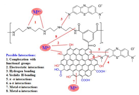
**Figure 14.** Illustration of possible mechanisms of pollutants–adsorbent interactions for the adsorption of metal ions and organic dye. (Note: some of the repeated or predefined interactions were for simplicity omitted, and M refers to metal ions).
