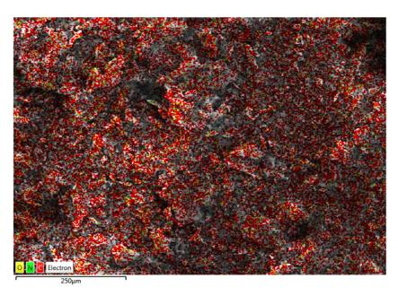
$\label{eq:figure 3.} \textbf{Mapping image indicating a uniform distribution of the N (from polyethyleneimine) among O and C in PEI/GO.}$
