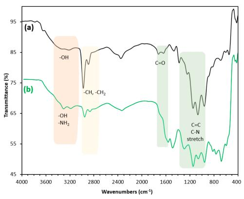
Figure 5. Fourier-transform infrared (FTIR) spectra of (a) graphene oxide and (b) PEI/GO.
