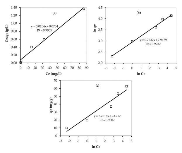
**Figure 12.** Linear isotherms of  $Pb^{2+}$  adsorption over PEI/GO: (a) Langmuir; (b) Freundlich; and (c) Temkin models. (pH = 6, PEI/GO dosage = 0.1 g, and 23  $^{\circ}$ C).
