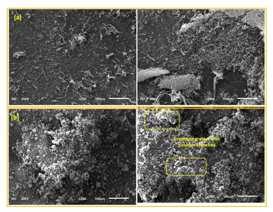
Figure 2. Scanning electron microscopy (SEM) images of (a) graphene oxide and (b) PEI/GO.
