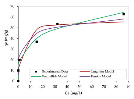
**Figure 11.** Nonlinear isotherms of  $Pb^{2+}$  adsorption over PEI/GO. (pH = 6, PEI/GO dosage = 0.1 g, and 23 °C).
