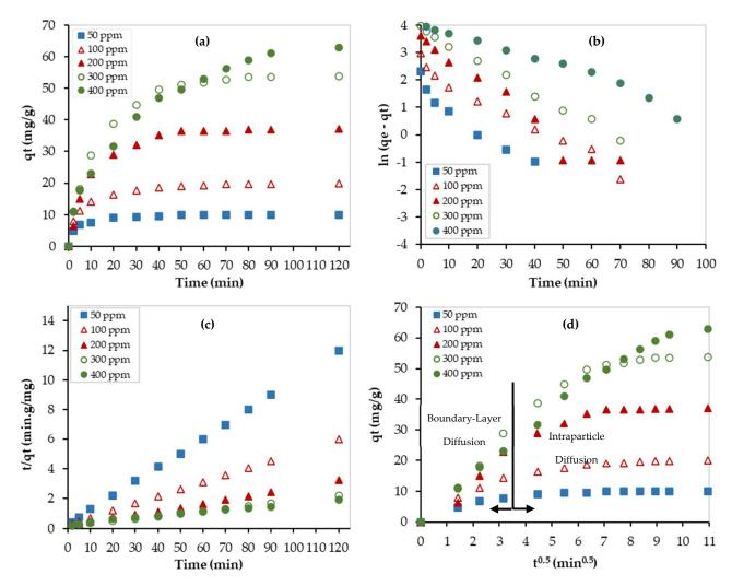
**Figure 9.** Kinetic studies for the  $Pb^{2+}$  removal using PEI/GO: (a) experimental data, (b) linear pseudo-1st-order model, (c) linear pseudo-2nd-order model, and (d) Weber–Morris model. (pH = 6, PEI/GO dosage = 0.1 g, and 23 °C).
