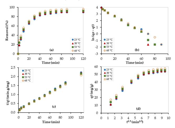
**Figure 10.** Kinetic studies for the Pb<sup>2+</sup> removal using PEI/GO at different temperatures: (a) adsorption capacity, (b) pseudo-1st-order model, (c) pseudo-2nd-order model, and (d) Weber–Morris model. (pH = 6, PEI/GO dosage = 0.1 g, Pb<sup>2+</sup> concentration = 300 ppm).
