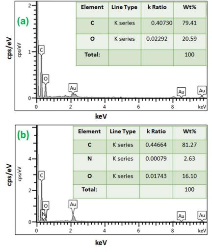
**Figure 4.** Energy-dispersive X-ray (EDX) spectra of (a) graphene oxide and (b) PEI/GO.
