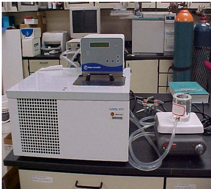
Figure 3-1. Bench-Scale Unit used for the Ferrate Preparation
