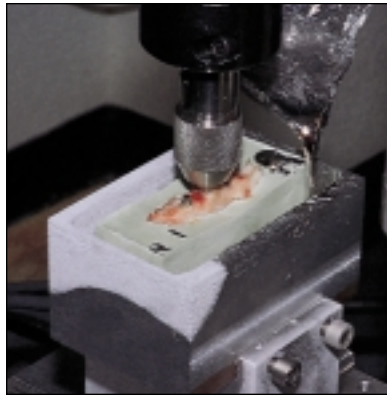
Fig 3a One specimen with three implants is embedded in dental cement and attached to the actuator, guaranteeing a perfect implant-actuator alignment. The implant-bone-dental cement complex is now affixed to the tub by filling in low temperature melting metal alloy.
