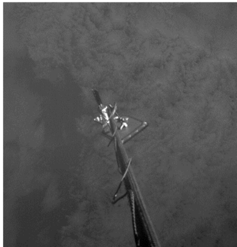
Figure 24. Target retained by harpoon tether wrapped around the boom.
