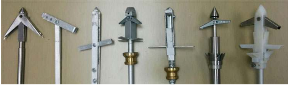
Figure 19. Harpoon tip and barbs design iteration.
