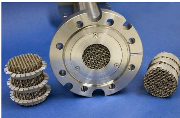
Fig. 4 Package tube. After a cleaning procedure, the structured package material is filled into the package tube inside a clean-room
