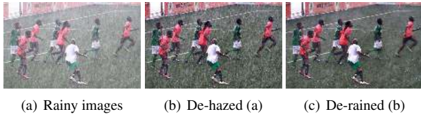
Figure 9: An example of heavy rain removal with dehazing.
