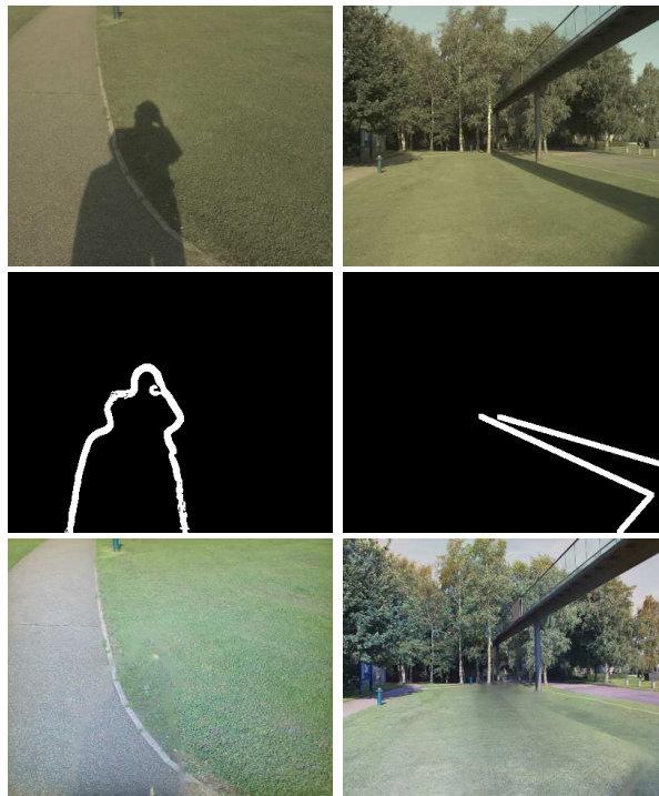
Figure 2: Original image (top), selected shadow edges (middle) and output images with shadow removed (bottom) for two images.
