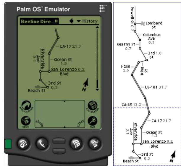
Figure 13: LineDrive map on a PDA. The route is rotated so that it fits the horizontally constrained image size of the PDA. The vertical dimension is unconstrained and users can scroll up to see the remainder of the route. This is the same route shown in figure 2.
