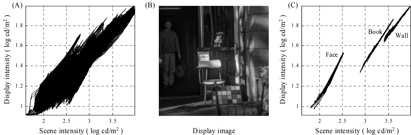
Figure 6. Tone reproduction operators are context-sensitive. Depending on its position in the image, a given intensity level may map into a different output level. (A) The distribution of input and output levels. (B) The output image. (C) The image to display intensity mapping of the TRO is illustrated for three different spatial regions of the image.
