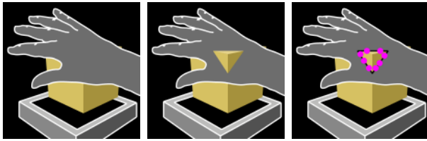
Figure 9: Hand-object intersection sampling. a) The hand in the scene touching the virtual cube with the ultrasonic transducer array position shown below it. b) The hand is converted into sixteen planes, some of which intersect the object in the scene, cutting the hand. c) The hand-object intersections are found as line segments and processed into contiguous arcs, from which control points are derived.
