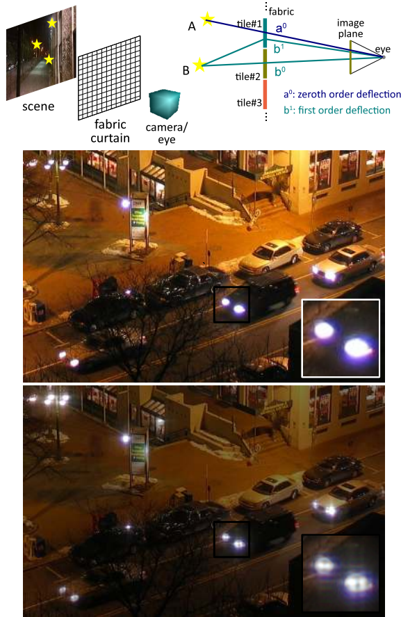
Figure 1: Effects created by a window fabric due to diffraction. (Top left) Looking at a scene from behind a fabric with fine tiled pattern. (Top right) Our framework predicts zeroth, first, and higher diffraction orders for intricate patterns. We model the fabric as tiled gratings and render diffraction from each tile independently. (Middle and Bottom) Rendering without and with the fabric. Notice the effects around bright sources.
