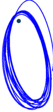
Figure 5. EML2 Southern NRHO with r_p = 5,930\text{km} , from multiple-shooting correction, after \sim 100 days.
