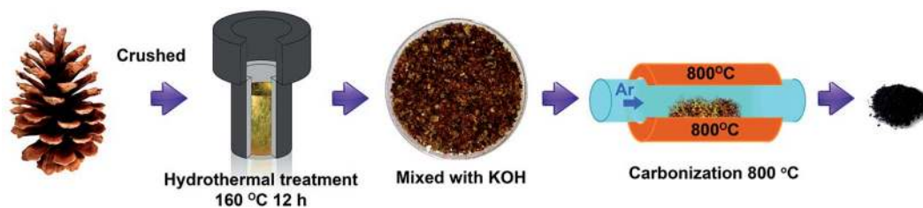
Scheme 1 Schematic diagram for the synthesis of porous carbons from pine cone.
