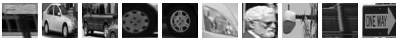
FIGURE 4 | The 10 shape prototypes used in conjunction with CT to encode the ROIs comprising the scenes (see section 7.1). Each ROI detected in a scene was represented by a 10-dimensional vector of its respective similarities to these 10 images.
