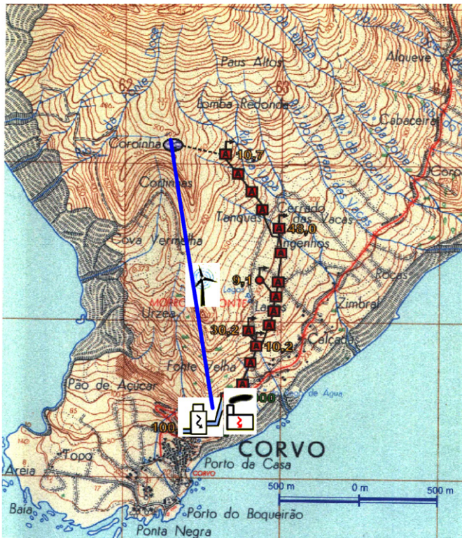
Fig. 3. The hydro-pumping storage system proposed for Corvo Island.
