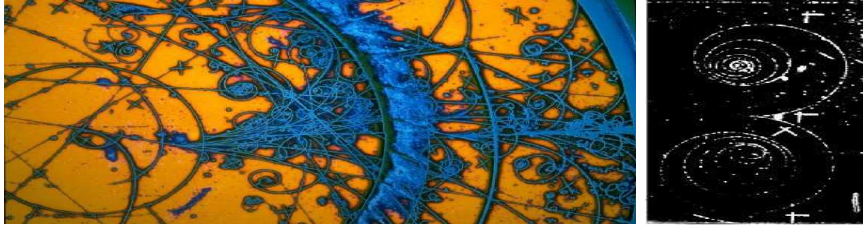
Figure i.2 : Tracks drawn by particles in a detector called bubble chamber. On the r.h.s. is a close-up of the central region, where a particle and antiparticle spiral in opposite directions.
