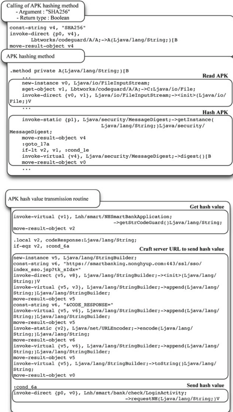
Fig. 5 APK integrity checking routine used in the N-bank app. It hashes the APK file using the SHA-256 hash function and sends the hash value to the designated URL
