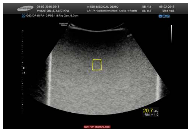
Fig 2. Samsung (S-SWE). Samsung S-Shearwave Elastography assessed on liver fibrosis phantom 3. The yellow box (centre) represents the shear-wave measurement area. ROI and the RMI (Reliability Measurement Index) is expressed below the obtained elasticity measurement of 20.7 kPa.
