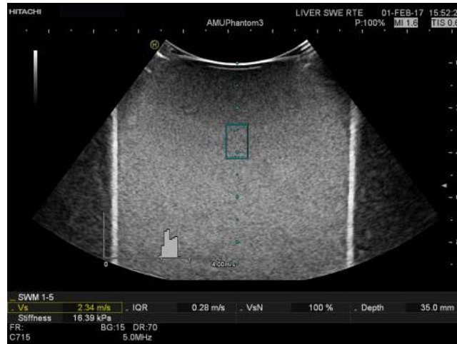
Fig 3. Hitachi (SWM). Hitachi SWM was applied on liver fibrosis phantom 3. The ROI is represented by the blue box (centre). The shear wave velocity measurements are presented in the histogram, and the median is given as Vs in m/s. Stiffness is based on this value expressed in kPa as well as the IQR (m/s), VsN (Reliability Index for shear wave velocity measurement) and the depth of the sample.
