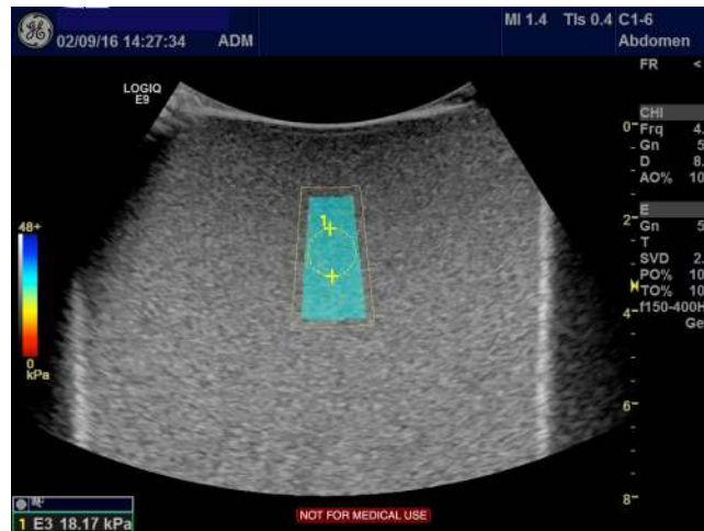
Fig 1. GE 2D-SWE. The figure illustrates the method of 2D-SWE by GE performed on liver fibrosis phantom 3 with Young’s modulus 24.8 kPa \pm 5%. The color box (centre) represents the elastogram, and the circle represents the ROI where the elasticity measurement is acquired. The blue color indicates harder tissue, as semi-quantitatively presented by the color scale to the left.
